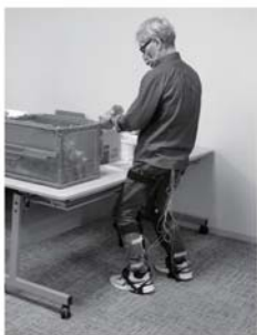
EMG measurement while standing works
